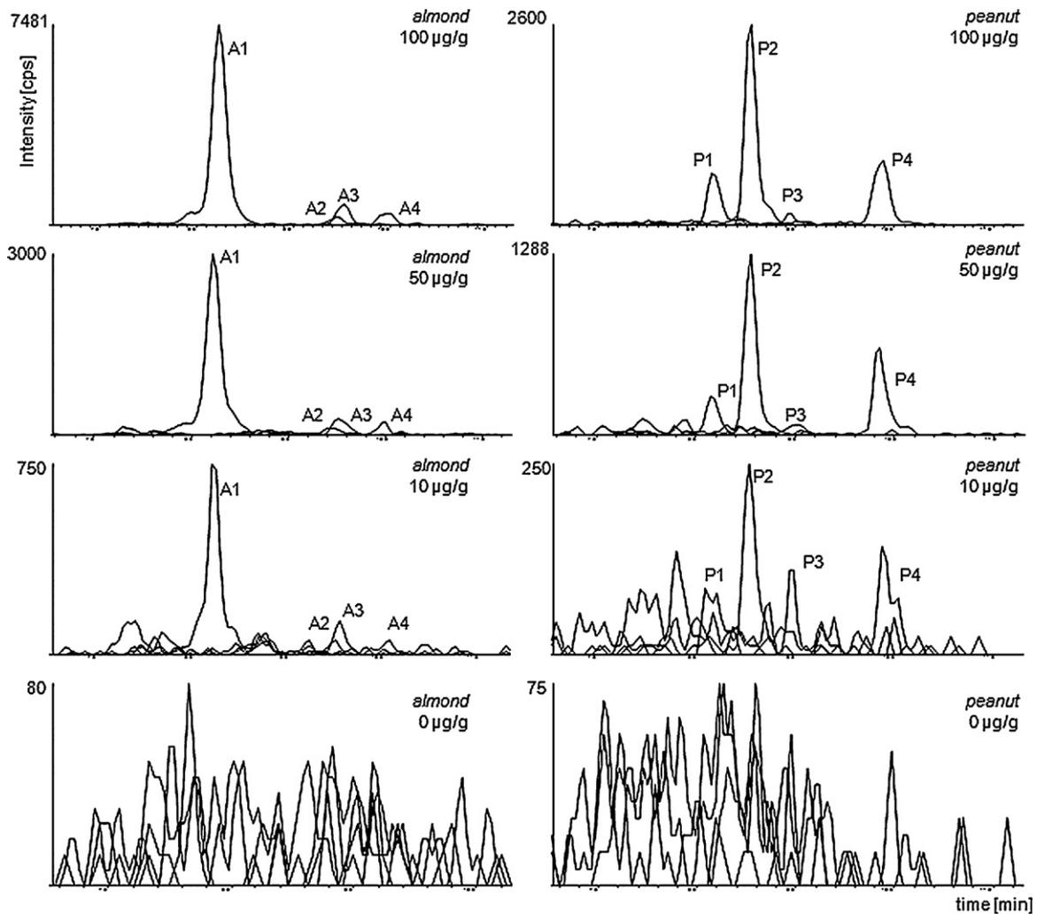
Fig. 3. Extracted MRM transitions for almond and peanut measured from different concentrations of the incurred bread material. The signals correspond to the following peptides: almond: A1: GNLPVQPPR, A2: GVLGAFSGCPETFEESQSSQGR, A3: ALPDEVLANAYQISR and A4: NGLHLPYSYNAPQLIYVQGR. Peanut: P1: DLAFPGSGEQVEK, P2: RPFYSNAPQEIFIQQGR, P3: GTGNLELVAVR and P4: WLGLSAEYGNLYR.
