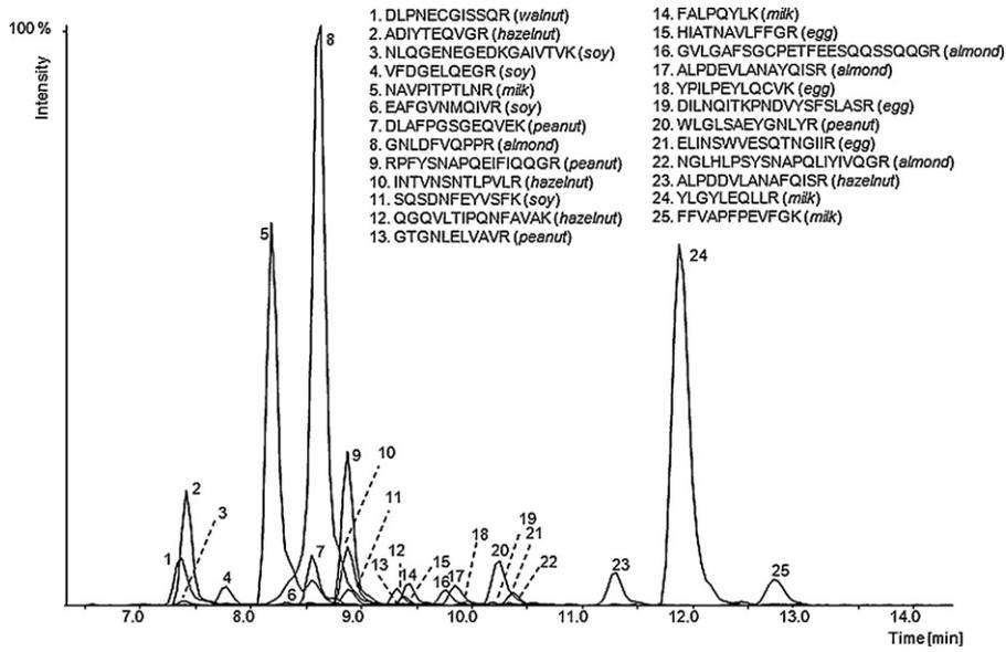
Fig. 2. MRM transitions for the incurred bread reference material containing 1000 ppm of all seven allergenic foods.
